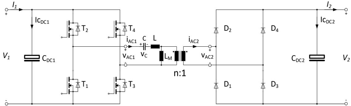
Figure 2 Principle Schematics of Isolated Unidirectional DC/DC Converter
