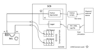
Figure 4. Scoreboarding XML transaction stream from external device, compare against REF.
