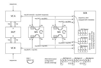
Figure 1. DUT, trailing models and scoreboard architecture. Bi-directional information flow on DUT ports. Configuration suitable for SoC bus interfaces.
