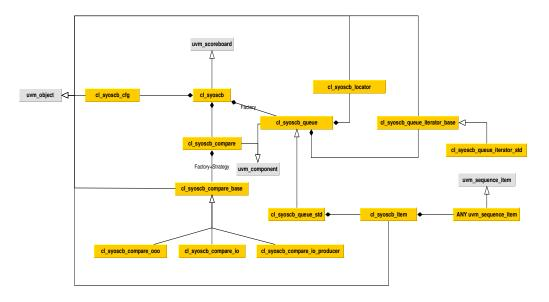
Figure 5. UML diagram: Scoreboard Classes.
