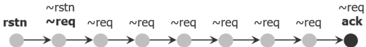
Figure 1: Safety property CEX, showing an 'ack' without a 'req'
