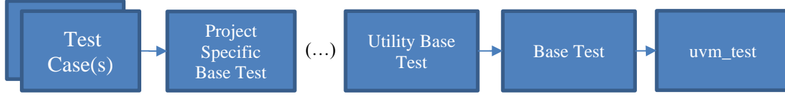
Figure 1. An example test hierarchy in a UVM compatible testbench
