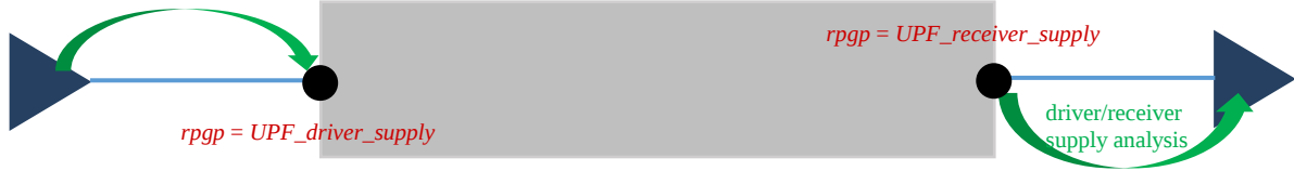
Figure 3: Driver/receiver supply analysis at top level with black-boxed block
