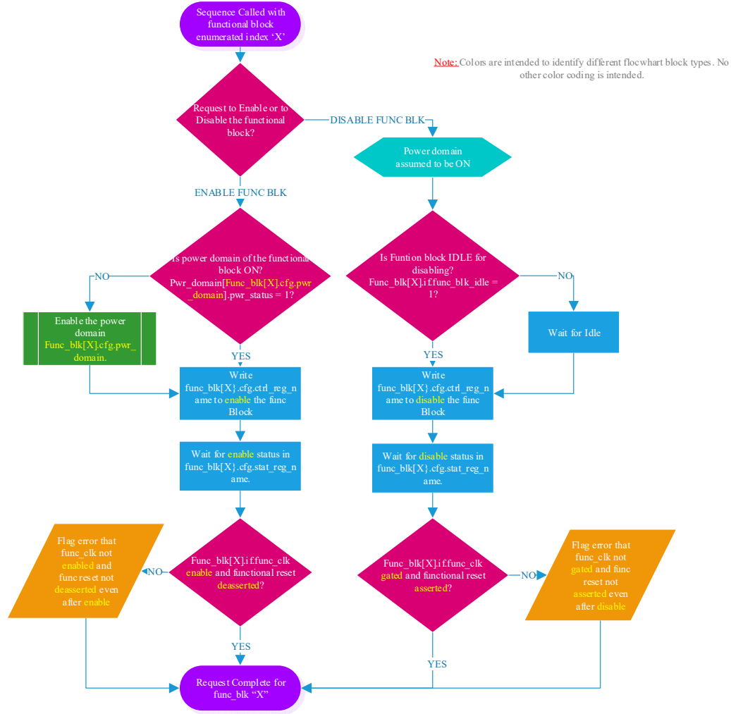
Figure 9: Flowchart for Function Block enable/disable sequence
