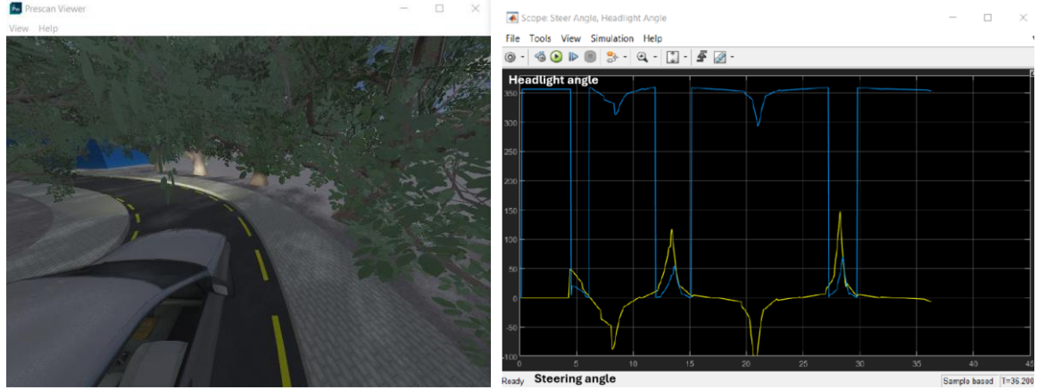
Figure 6. Application Use-Case (Adaptive Headlight) - Scope of Steering Angle Vs. Headlight Angle values from Simulink
