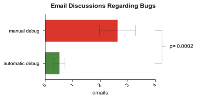
Figure 10. Comparison of the number of emails concerning test failures after manual and automatic debug. A statistically significant difference ( p=0.0002 ) between manual and automatic debug was found. With manual debug there are 5 times more emails discussing failures compared to automatic debug.
