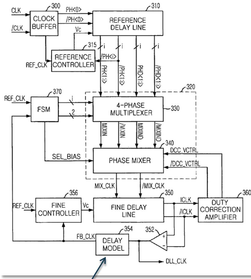
Process/temperature/voltage sensitive delay
