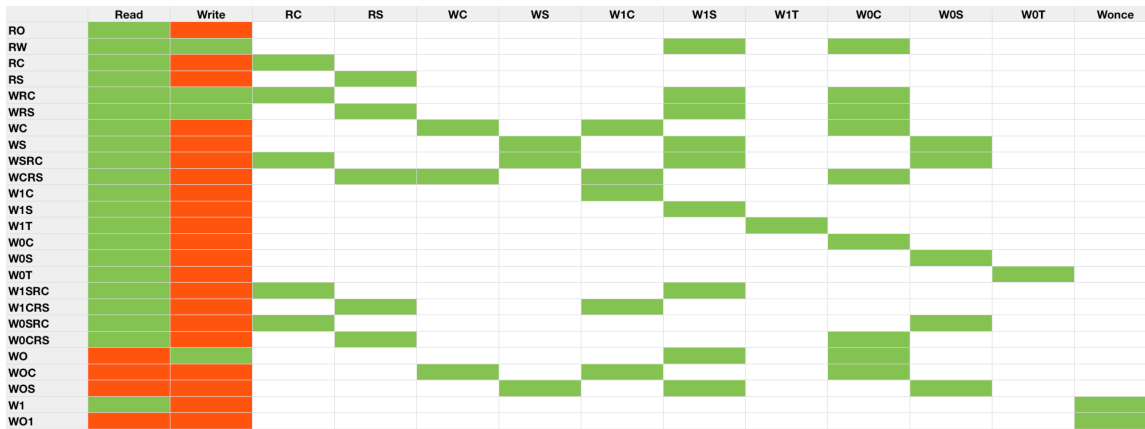
Figure 11. A decision table to determine the best access policy from UVM-based back-door exploration results (Columns correspond to each exploration property as conditions. Rows correspond to the UVM predefined access policies as determined policies. If a cross section is green, proof is expected for the condition property. If it is red, violation is expected. If it is white, the condition is don't-care.)
