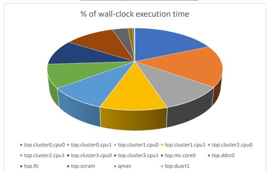
For one of the software workloads, the profiler helped uncover that one of the UART model instances was consuming most simulation time, which was both undesirable and unexpected. But having this uncovered, it was simple to fix the issue by removing the unnecessary synchronization requirement enforced by the model and help improve simulation performance by around 200%.
