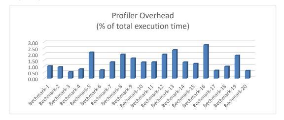
The measured overhead of the in-built profiler across a range of 20 benchmarks was less than 1.5% on an average and approx. 2.8% in the worst case.
