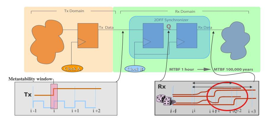
Setup Violation: Transition at input of synchronizer will propagate to output after **2 or 3** active edges of Rx clock in silicon
