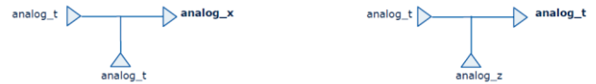
Figure 5: Resolution function examples used in the analog_pack package for modeling and simulation support.
