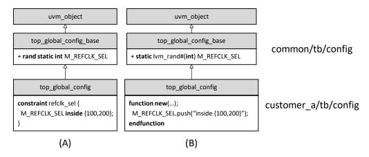
Figure 5: Top global configuration object structure defined in common directory, extended to customer project.
