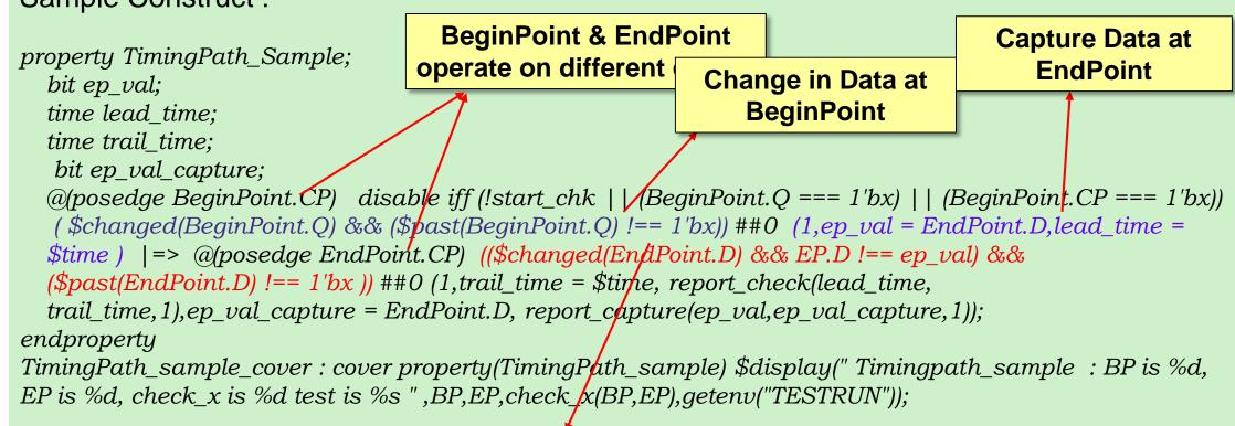
Wait for change in Data at EndPoint at the nearest edge of EndPoint clock after BeginPoint clock edge
