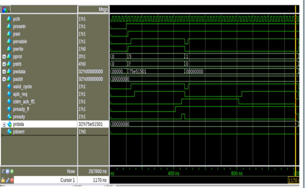
The figure below shows the handshaking taking place taking place between the two clock domains.
