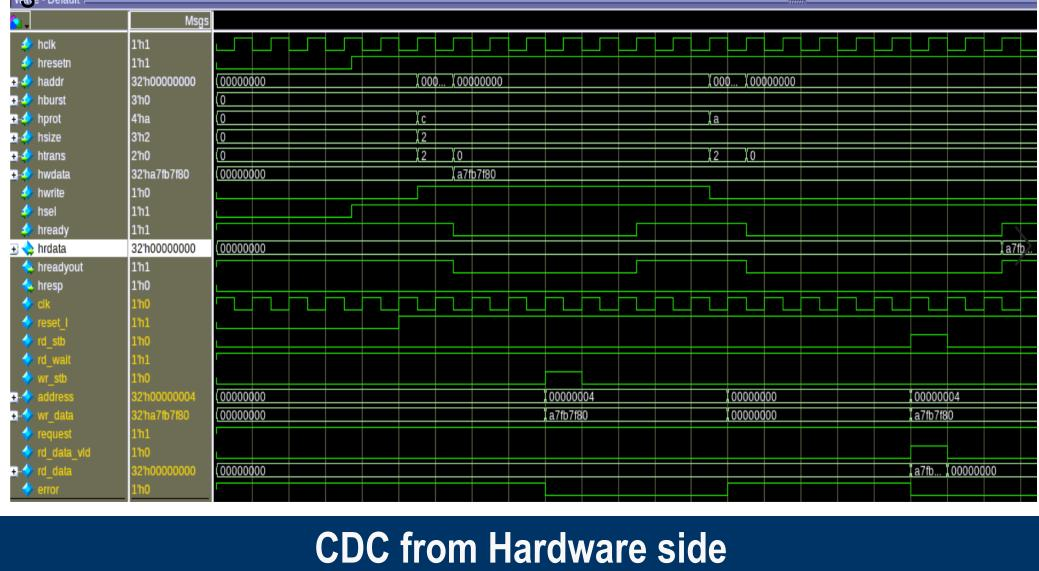
In the diagram shown below, two clocks one coming from bus (say APB) on which read write are will take place on register bank from software side and the other one is user define clock(CLK\_2) on which hardware side will do the read/write operation on the register bank. The handshake synchronizer is used to translate the transaction coming in from CLK\_2 domain to APB\_PCLK domain.
