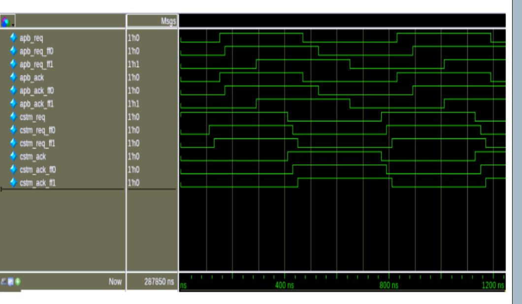
The figure below shows the CDC at the custom bus domain side, where when APB acknowledge is received, for the write transaction, the data write strobe and address are obtained.
