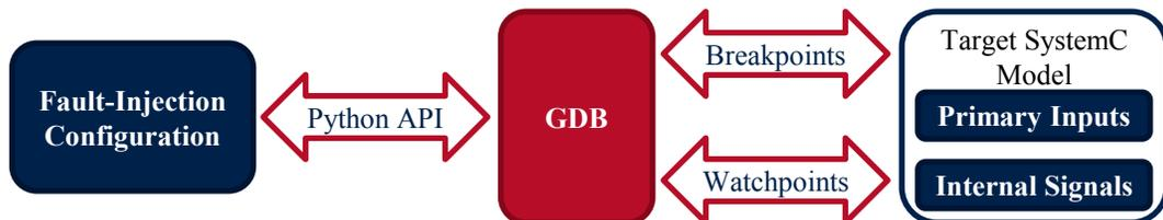
Figure 3. SCFIT's fault-injection mechanism
