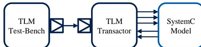
Figure 7. TLM transactor which controls the SystemC representation of a gate-level model
