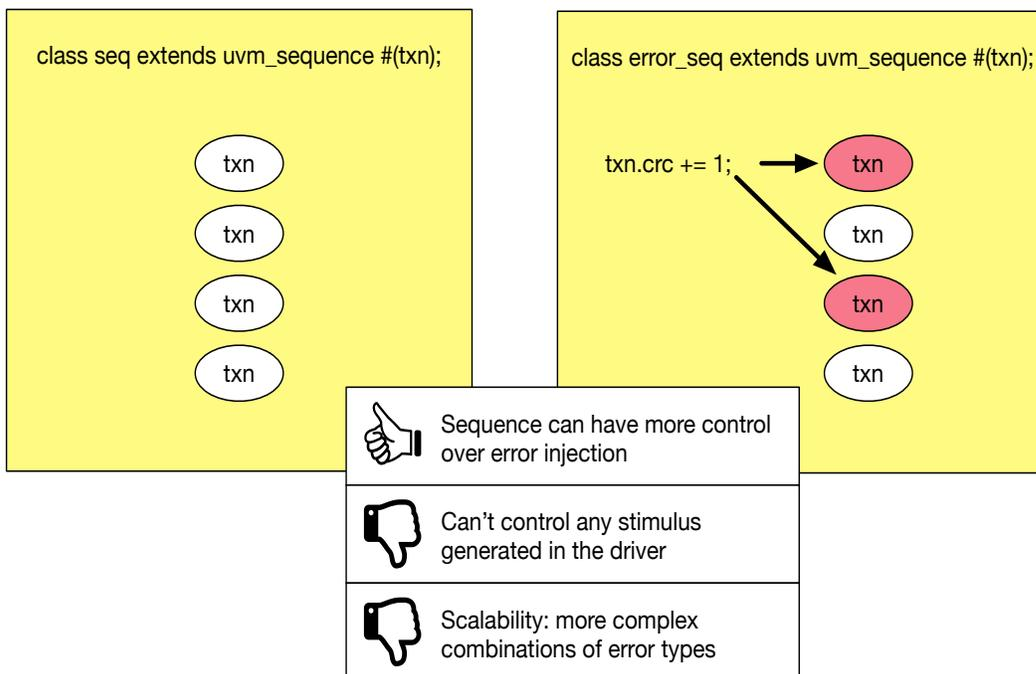
Figure 2. Error injection in a sequence.
