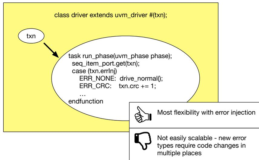
Figure 3. Error injection in driver.
