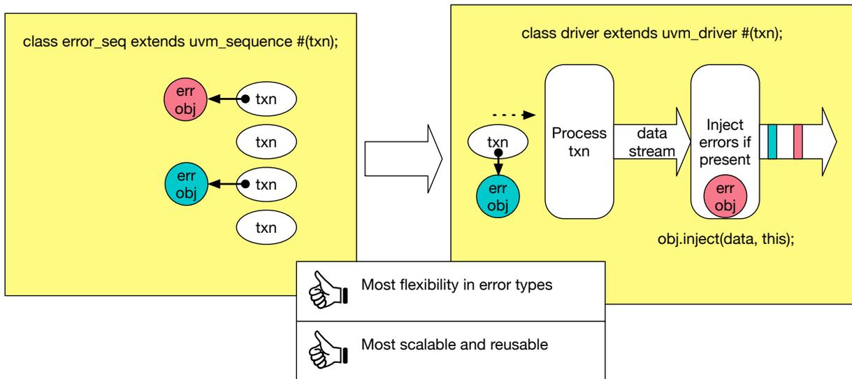
Figure 4. Error injection with error objects.
