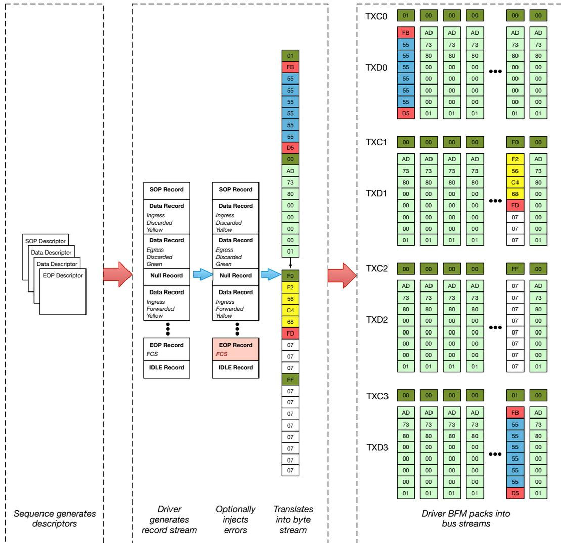
Figure 6. Overview of object-based error injection strategy.
