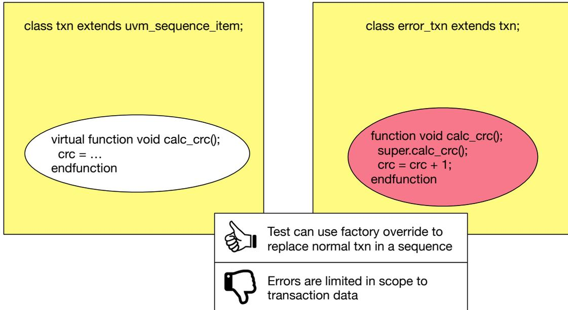
Figure 1. Error injection through transaction class extension.
