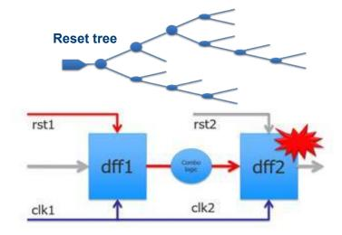
If rst1 is asserted while rst2 is not asserted, the asynchronous data from dff1 will metastability on dff2
