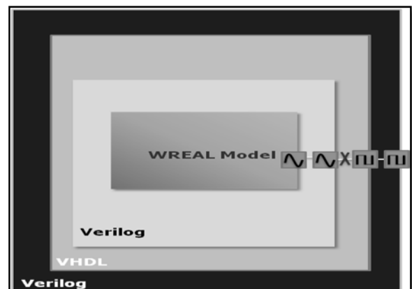
Fig. 6: Stopping coercion at VHDL using ‘rnm_coerce’
