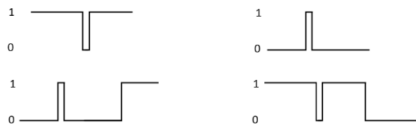
Fig 1: Examples of glitches on combinational logic
