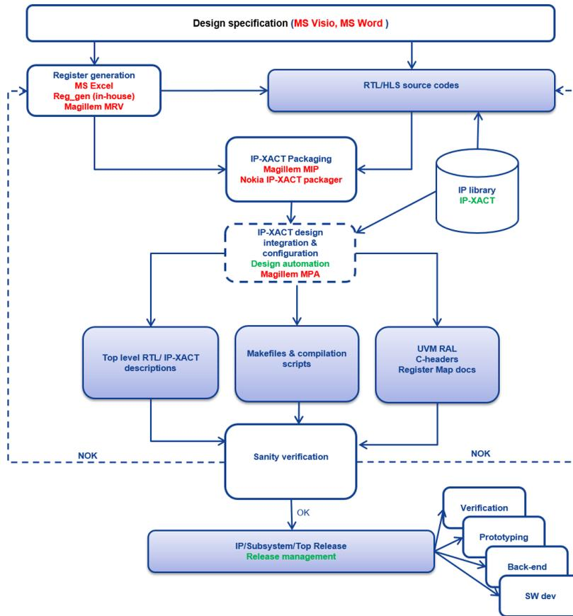
**Figure 1 - High-level view of the Nokia SoC Design Flow**
