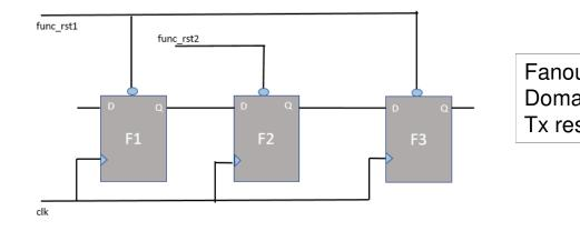
func\_rst2 func\_rst1 POR func\_rst1 F1 F2 clk Fanouts of Rx Flop(F2) transmits to Tx Reset Domain (func\_rst1) Tx reset assertion blocks metastability transmission
