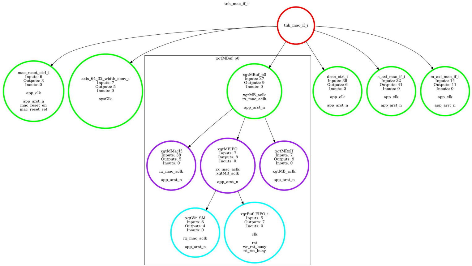
Diagram 1: tnk_mac_if block diagram (image generated using graphviz)
