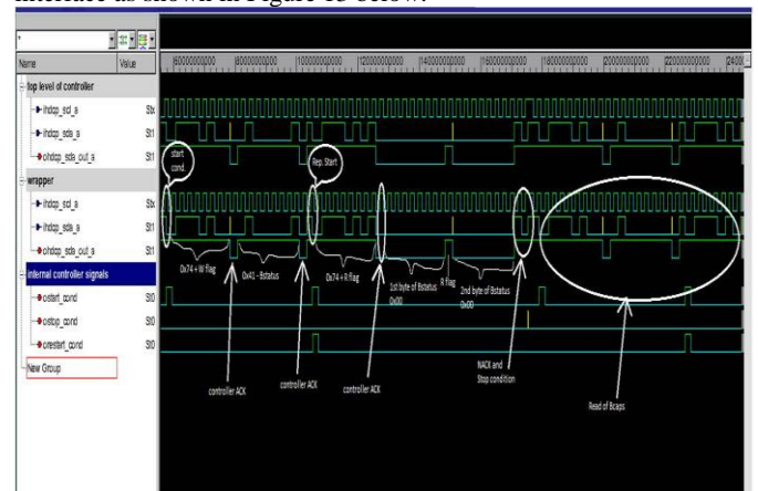
Figure 13: HDCP sequence as viewed on the DUT ddc interface
