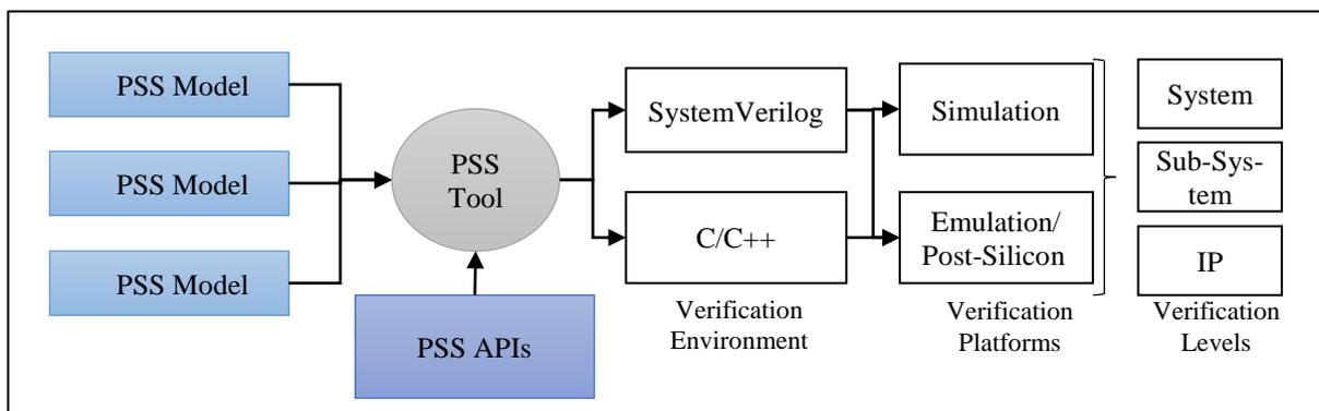
PSS helps describe test intents at an abstract, test-implementation agnostic level. This test intent, also called a scenario, can be used later to run the same or extended configuration on various platforms like simulation,
