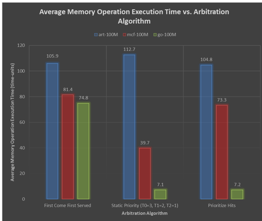
Figure 21: Plot of Average Memory-Access Latency vs. Arbitration Algorithm for Test-Scenario 6
