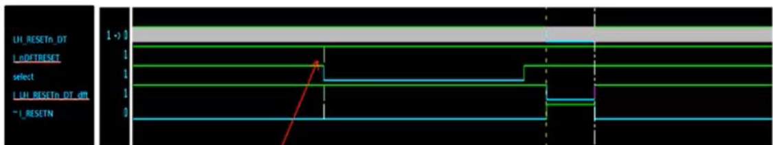
Glitch introduced and propagating through the design
