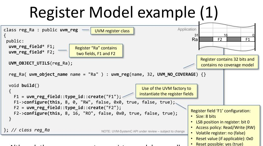
Although the user can create a register model manually, the recommended use model is to generate this register model from an IP-XACT register description
