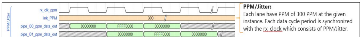
Figure 4. PPM/Jitter – Sample Waveform showing clock with PPM + Jitter
