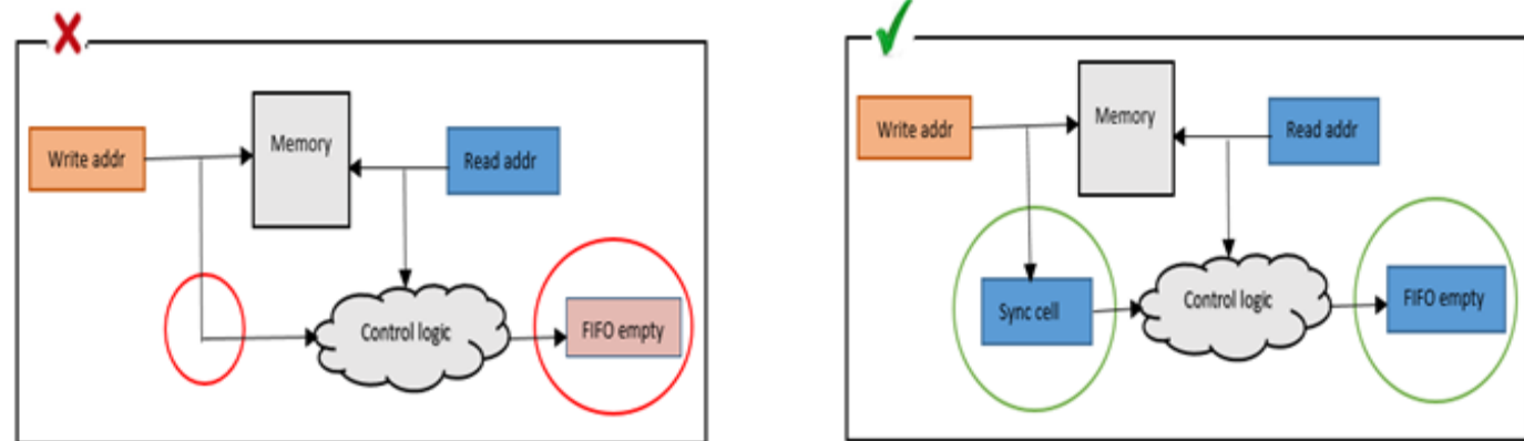
Risk of using unsynchronized write address for generating FIFO empty
