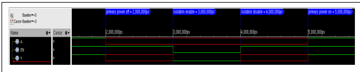
Figure 8. Correct simulation waveform snapshot of the enable level-shifter
