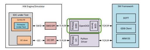
Info : SWD DPIDR 0x0bc11477 Info : cortex m0p sim: hardware has 4 breakpoints, 2 watchpoints Info : starting gdb server for cortex\_m0p\_sim on 3333 Info : Listening on port 3333 for gdb connections Info : accepting 'telnet' connection on tcp/4444 target halted due to debug-request, current mode: Thread xPSR: 0x01000000 pc: 0x20000180 msp: 0x20000508
