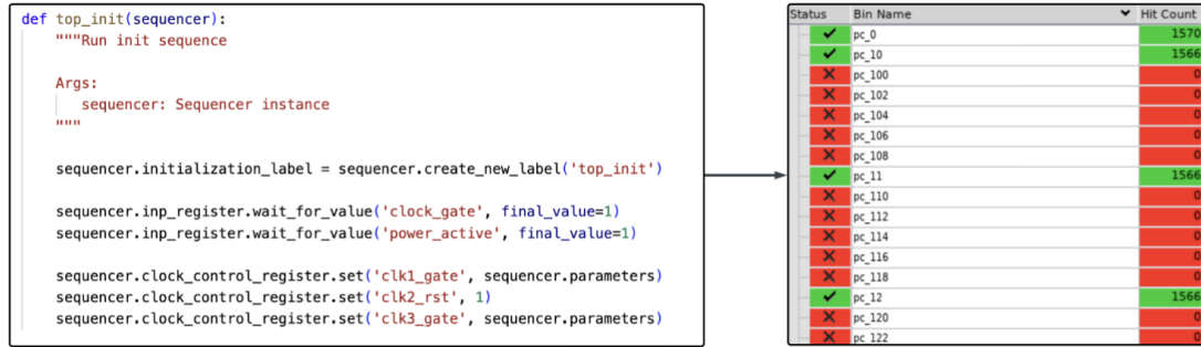
Figure 2: Intelligible Source Code (left) vs. Opaque PC Coverage Data (right)
