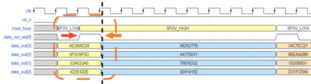
Fig. 7. SR8 simulation waveform after RTL weakness insertion
