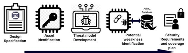
Fig. 2. Security Verification Plan
