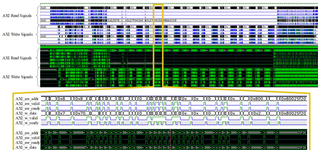
Figure 3. Waveforms of read and write AXI bus transfers for SystemC (white background) and RTL platform (black background) of Dhrystone benchmark with 10 runs;
