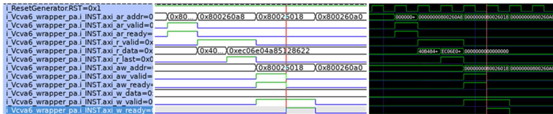
Figure 4. AXI waveforms of single read and write bus transfers in SystemC (left) and RTL (right)
