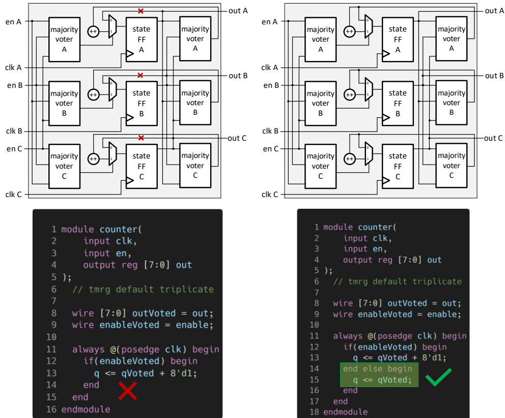
Figure 13 Illustration of a bug in a simple counter due to the omission of an else condition by the designer is shown on the left. Although this circuit produces functionally correct output under normal conditions, it lacks protection against SEUs. When the enable signal to the counter is held low, an SEU in one of the state flip-flops cannot be corrected. If another SEU occurs in a different state flip-flop while the enable signal remains low, the circuit will produce an incorrect output.
