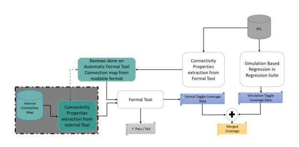
Fig. 2: Formal and Simulation based Verification Flow for Coverage sign-off
