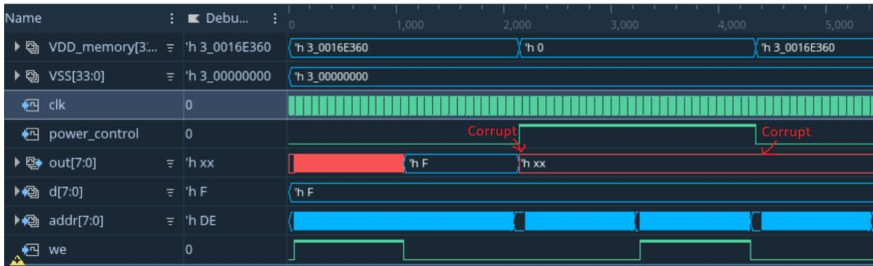
**Figure 7. Memory corruption results at power down with memory wrapper**
