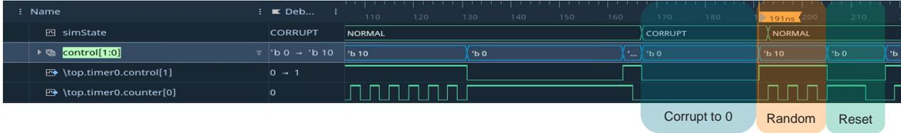
Figure 3. Emulation (2 State) showing 0 during power OFF and random after power ON
