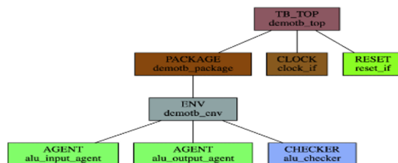
Figure 7. The testbench tree structure for a simple ALU generated by the web gui of Gingko
