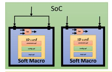
Macro synthesized as standalone block SoC reuses netlist of Macro regardless Both Instance of Macro have isolation cells
