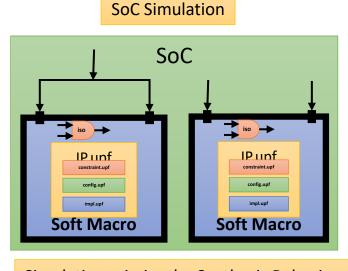
Simulation mimics the Synthesis Behavior Because of Soft Macro marking
