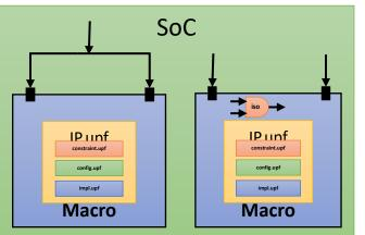
Simulation will not see Isolation Cell In the instance where supply is shorted
