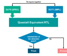
INPUTS DUT0 = Original RTL DUT1 = DUT0 with fault asserted
