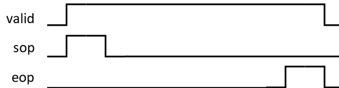
Figure 2: Packet handshake protocol.
